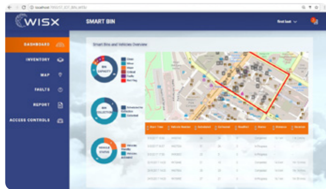
Dashboard view with bin sensors status and location detail, for more efficient and optimised cleaning schedule
